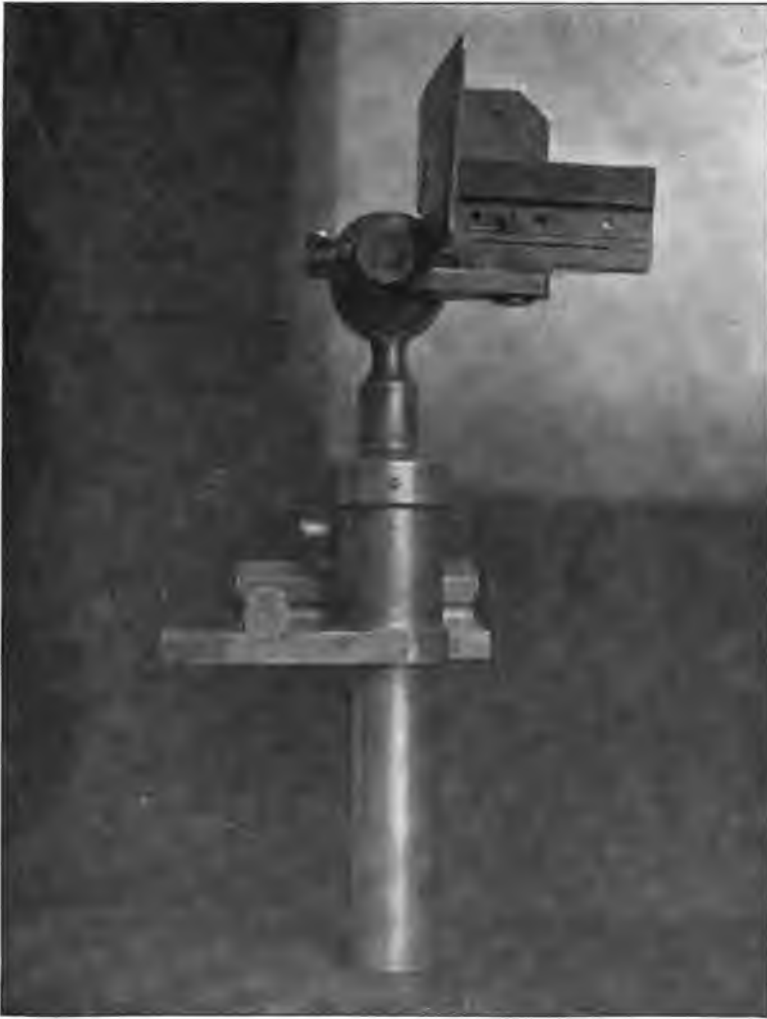
GONIOMETER (FRENCH) FOR TRAINING GUNS IN AZIMUTH.
